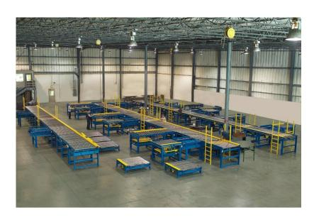
product from multiple packaging lines to the shipping and receiving area – not an ideal situation due to the congestion, high traffic intersections and potential hazards to workers. The customer wanted to reduce the fork truck traffic and still be able to transport the product to the loading docks from the same existing production lines.
