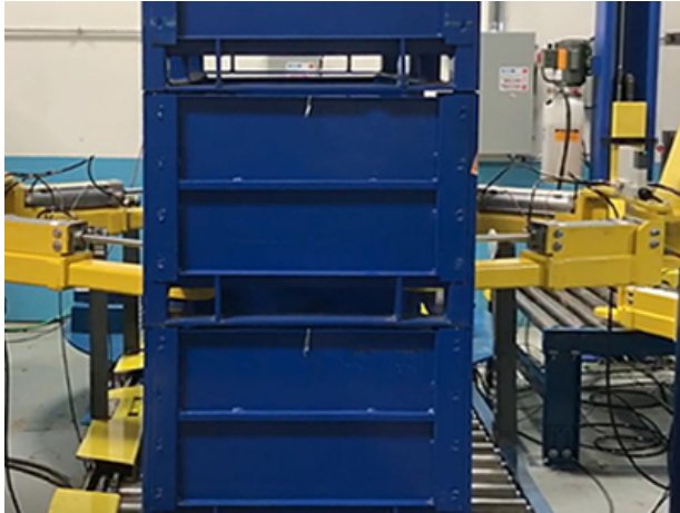
(Left) End view of Sun Volt Systems' Automated Robot destacking three totes. Totes weigh 200 pounds each. (Right) Close up shot of Sun Volt Systems' Automated Robot lifting arm.
