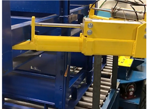
(Left) End view of Sun Volt Systems' Automated Robot destacking three totes. Totes weigh 200 pounds each. (Right) Close up shot of Sun Volt Systems' Automated Robot lifting arm.
