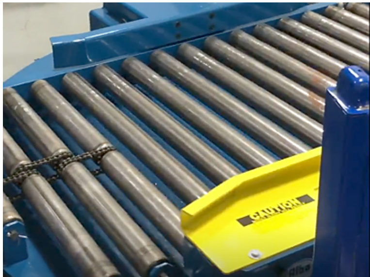
A pneumatic side pusher, mounted to the turntable's top plate, aligns the tote's leading edge before it enters the robotic, tube loading zone.
