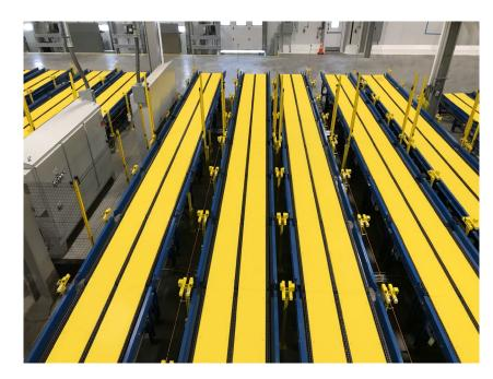
System). Alba designed the conveyors to bring the finished product to the storage system and supplied the conveyors to take the finished product back to the warehouse when ready for shipment.
