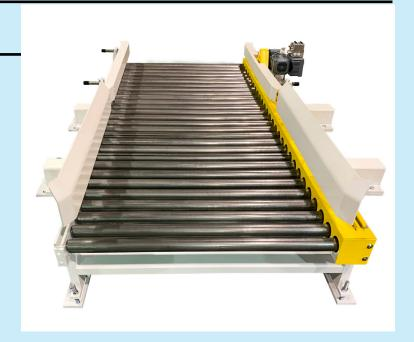
Alba provided CDLR conveyor and a frame-to-frame transfer for conveying the load. The integrator required special guide rails, end stops, and Unistrut to be mounted to the conveyor. The equipment was manufactured in Alba's plant in Fairfield, Ohio, then inspected, and shipped to the integrator for complete integration into the system.
