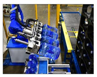
After Automated Motion releases the stack from the clamping frame, Alba's pallet conveyor then conveys the full pallet stacks to the downstream lift and rotate conveyor. This conveyor lifts and rotates the full stacks 180 degrees so the bottle necks now face away from the robot.
