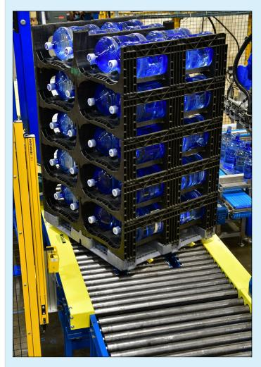
The rotation is important because the stack of full pallets is then removed from the conveyor from the side by fork truck. This same fork truck then transports the bottles ready to be loaded into a delivery truck with necks facing the fork truck driver. This allows the person delivering to homes and businesses to reach for the bottles by the neck and remove them by hand out of the pallet and place them onto a dolly for transport.
