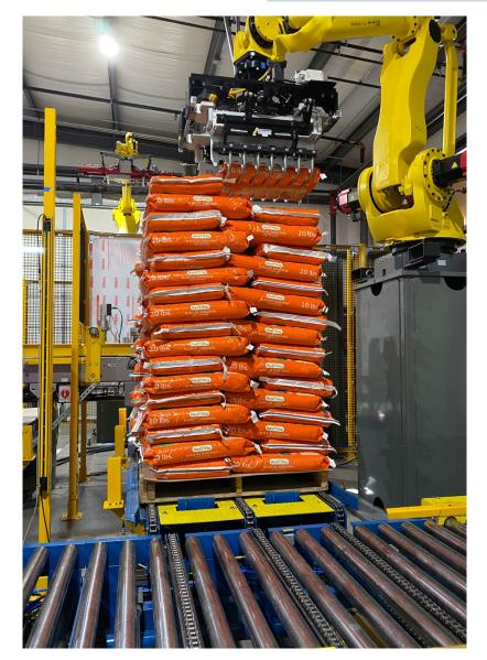
when loading the pallets with a robot. The pop-up chain transfers and CDLR conveyors are used for transferring the full pallets to the stretch wrapper and then to the fork truck pick-off area for pallet removal from the system.
